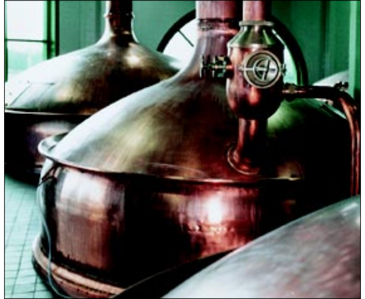
Approximately 11,000 lb (5,000 kg) of flat rolled copper were required to build the new kettles.
