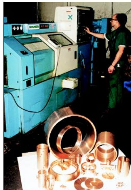
A selection of bearings and bushings and a modern NC Turning Centre.
